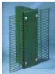
The Bekasecure post's design and high yield strength steel provide the ultimate in high security, rigidity and ease of installation. Posts are foreseen with a double range of wholes 10 x 20 mm and the fixation of the panels is secured by the use of a continuous cover plate and specific inox security bolts. The open profile of the post allows electrical or fibre optic cabling and is closed with specific metal cap.
